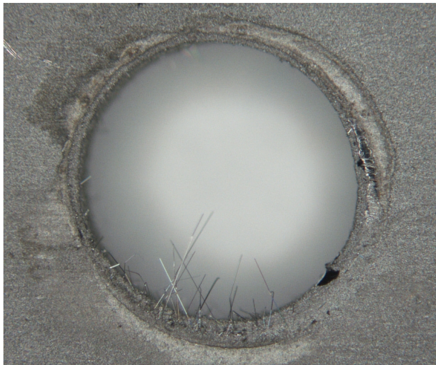
Figure 1 Tin whisker growing on the inside of a mounting hole
